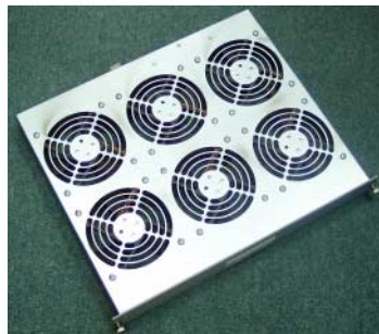
Figure 2-6 Outside view of the radiator fans
